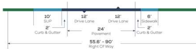
PROPOSED TYPICAL SECTION - ORION DR (GOODWIN LN - FM 1102)
