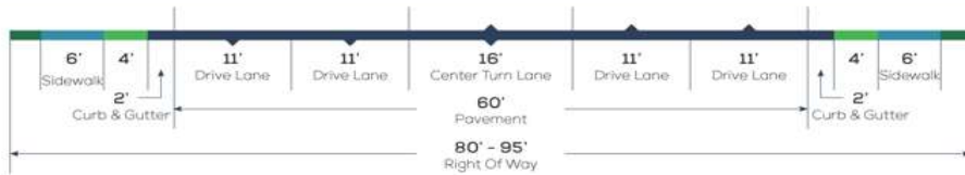
PROPOSED TYPICAL SECTION - COMMON ST (LOOP 337 - FM 306) SCALE: 1/8" = 1'
