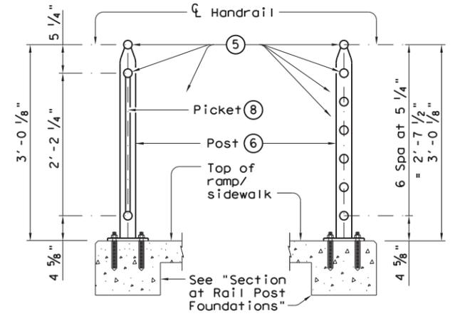
**SECTION C-C** (Showing Handrail TY C)
