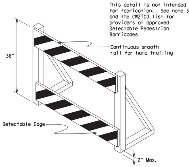
This detail is not intended for fabrication. See note 3 and the CWZTCD list for providers of approved Detectable Pedestrian Barricades
