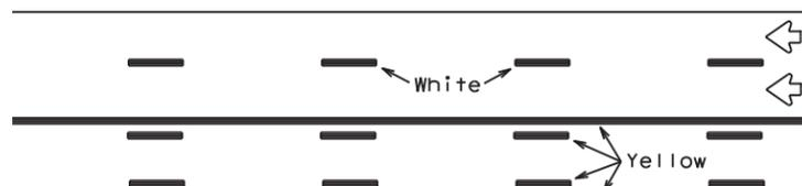
REFLECTORIZED PAVEMENT MARKINGS
