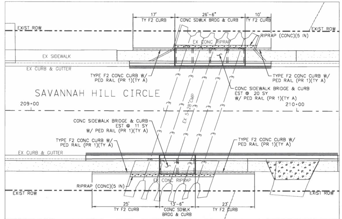
**SIDEWALK BRIDGE & TYPE F2 CONC CURB PLAN VIEW**
