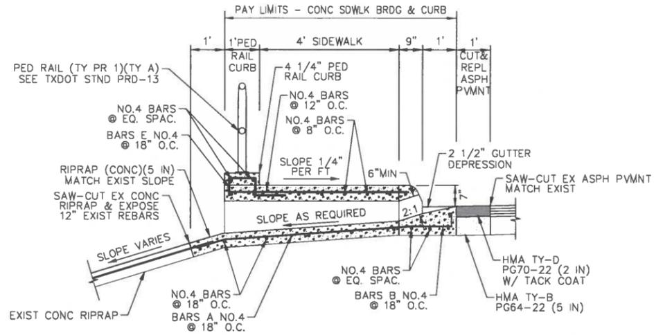
**CONC SIDEWALK BRIDGE & CURB SECTION VIEW**
