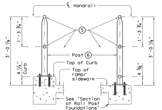
**SECTION A-A** (Showing Handrail TY A)
