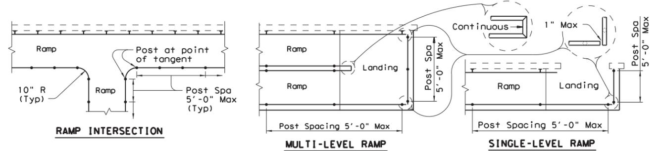
**PLAN SHOWING RAIL AT RAMP CONDITIONS**
