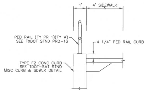
**TYPE F2 CONC CURB DETAIL AT BACK OF SIDEWALK**
